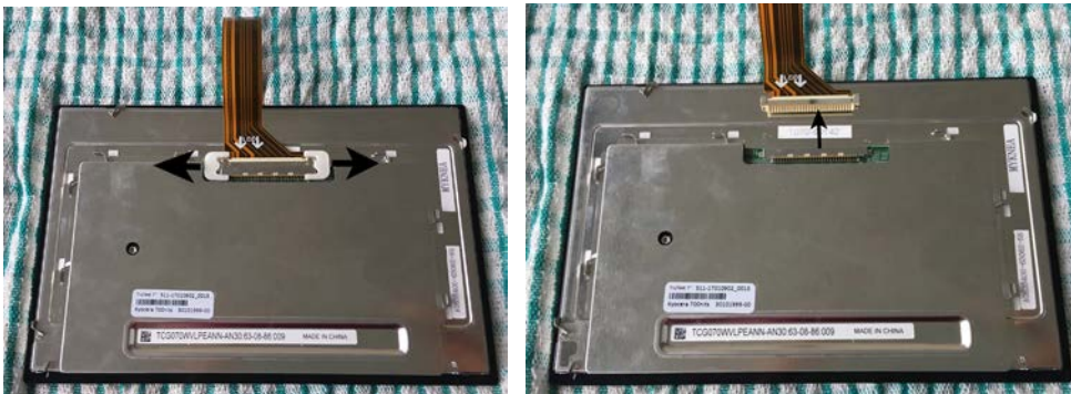
Figure 22: Removing the LCD connector clips and disconnecting the LCD FPC
