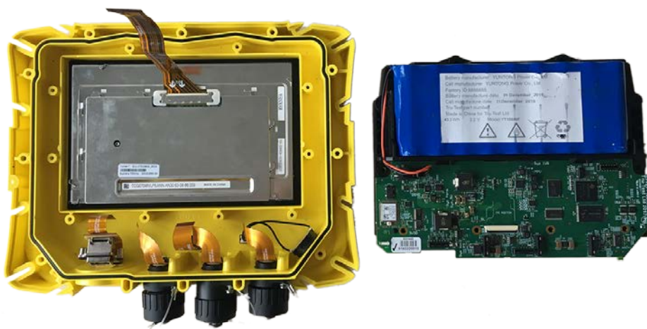
Figure 20: Removing the cradle assembly
