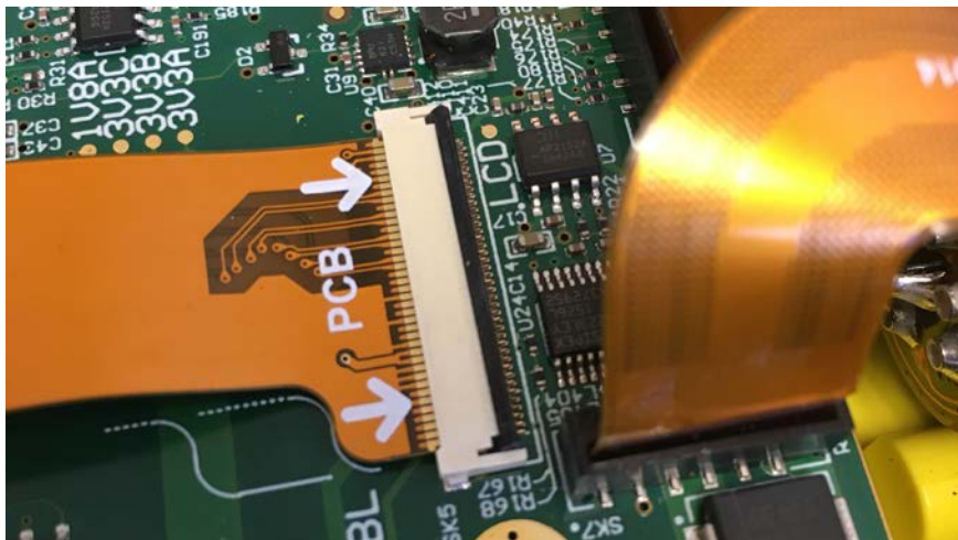
Figure 1: LCD FPC connector open
