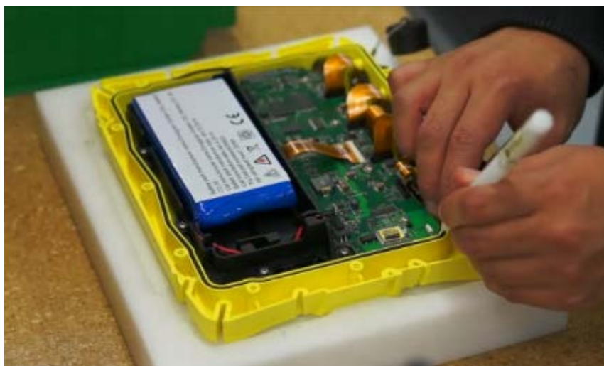
Figure 9: Using a plastic pen to press the o-ring into the groove at the corners.
