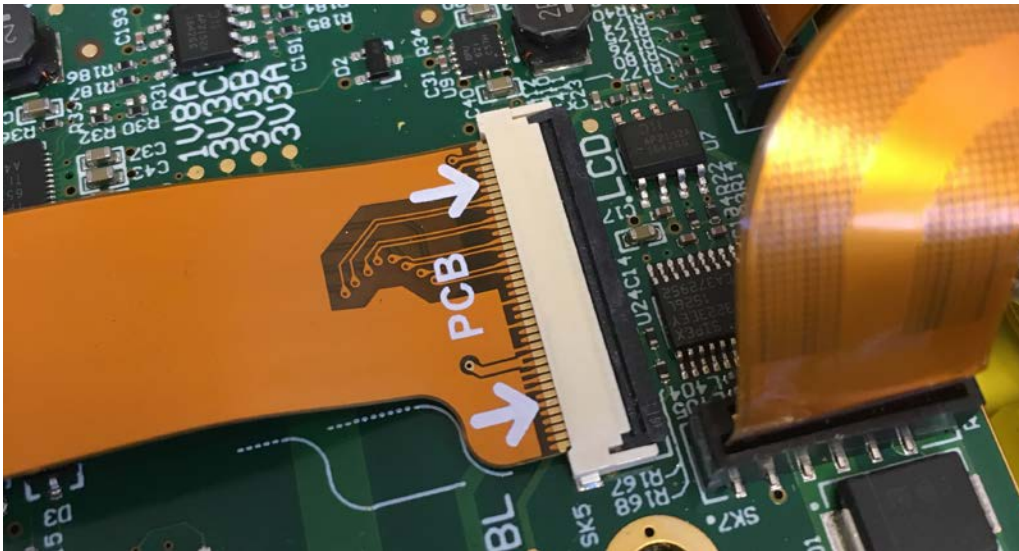
Figure 2: LCD FPC connector closed.
